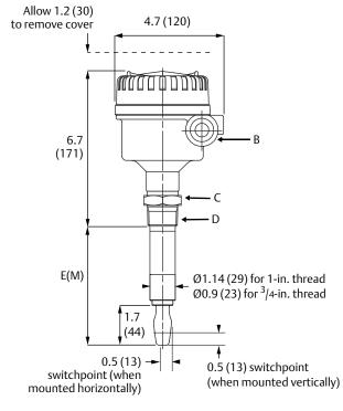
A. Cable entry M20 x 1.5 or  $^{1}$ /2-in. ANPT B. Cable entry M20 x 1.5 or  $^{3}$ /4-in. ANPT
