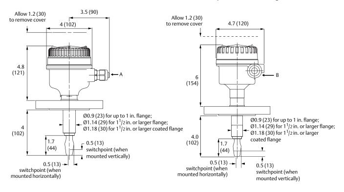
A. Cable entry M20 x 1.5 or  $^{1}/_{2}$ -in. ANPT B. Cable entry M20 x 1.5 or  $^{3}/_{4}$ -in. ANPT
