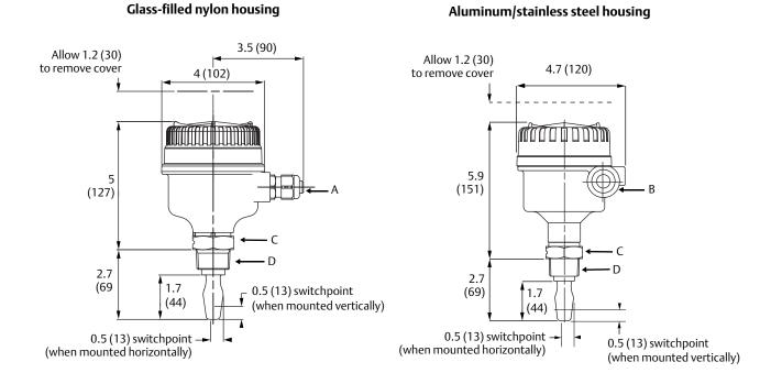
A. Cable entry M20 x 1.5 or  $^{1}/_{2}$ -in. ANPT B. Cable entry M20 x 1.5 or  $^{3}/_{4}$ -in. ANPT
