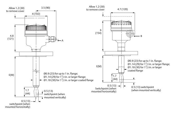
A. Cable entry M20 x 1.5 or  $^{1}/_{2}$ -in. ANPT B. Cable entry M20 x 1.5 or  $^{3}/_{4}$ -in. ANPT
