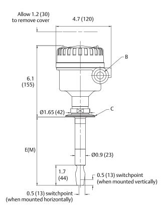
A. Cable entry M20 x 1.5 or  $^{1}$ /2-in. ANPT B. Cable entry M20 x 1.5 or  $^{3}$ /4-in. ANPT
