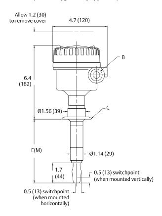
A. Cable entry M20 x 1.5 or  $^{1}$ /2-in. ANPT B. Cable entry M20 x 1.5 or  $^{3}$ /4-in. ANPT
