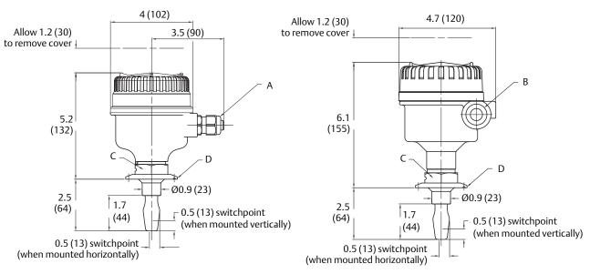
A. Cable entry M20 x 1.5 or  $^{1}$ /2-in. ANPT B. Cable entry M20 x 1.5 or  $^{3}$ /4-in. ANPT Dimensions are in inches (millimeters).
