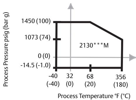
Figure 2. Operating Temperatures
